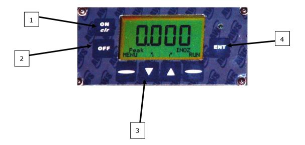
**Special Note**: MTMDP-2S PTEST is a modified version of the MTMDP series. The top line of the display shows the number of samples taken during a test. Pressing the ENT button at the end of 3 samples will bring the user to the results screen.
